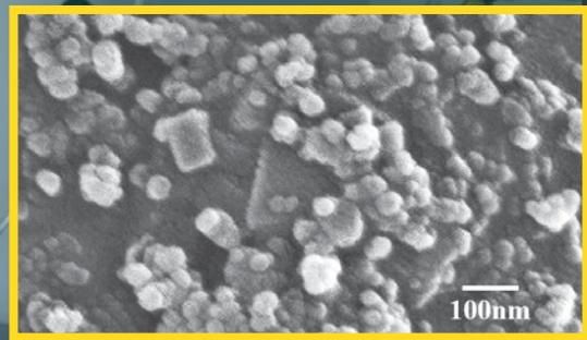
Dr. Hongyan Ma will test producing calcium carbonate nanoparticles inside highly diluted wet cement
